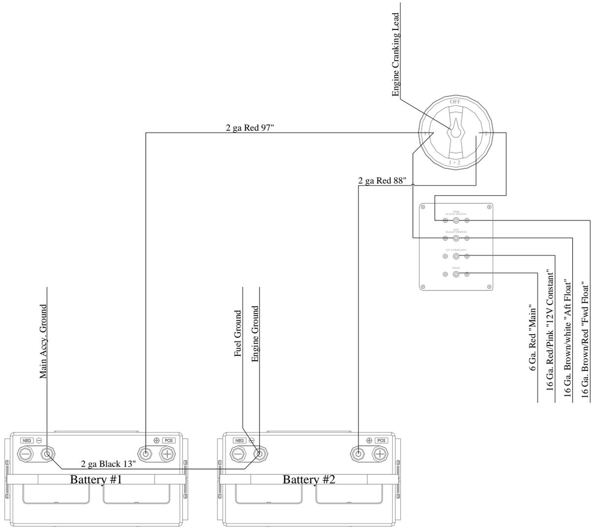
*Battery Wiring with Select Switches – Dual*
