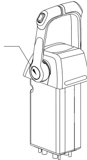
Reverse the shift mechanism to stop a boat that is moving forward. This change in direction will provide a “braking action” and slow the boat.
